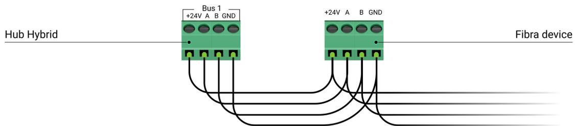
**+24V** – power supply terminal of 24 V<sub>DC</sub>.
