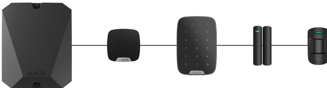
For the **Beam (Radial)** topology, be sure to install a 120 Ohm terminating resistor at the end of the line (included in the hub complete set). The terminating resistor is connected to the signal terminals of the last detector on the line.
