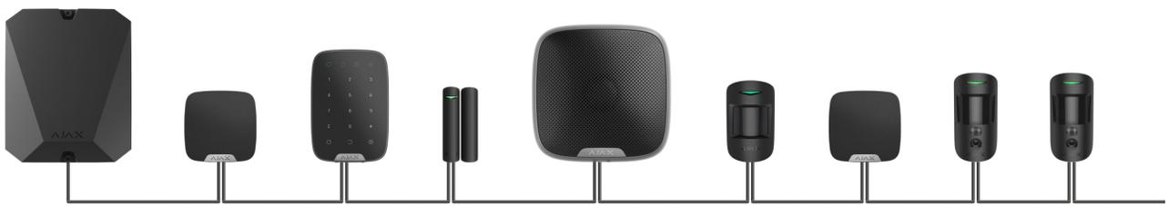
**Ring connection method** occupies two bus outputs of the hub. If the ring breaks in one place, no device will be disabled. The ring reconfigures into two lines, which continue to operate normally. Users and the security company will receive notification about the break.
